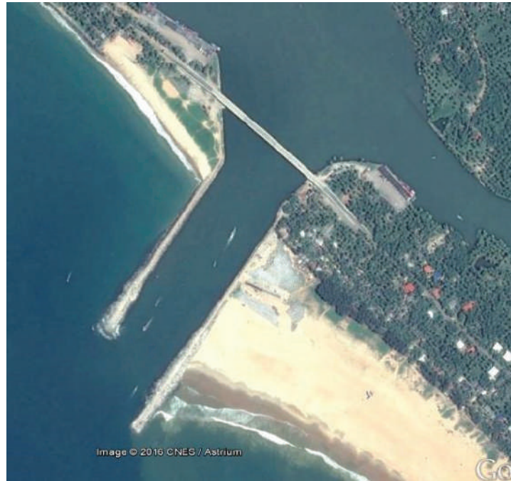
Fig. 5.4. Beach formation and erosion respectively on the south and north sides of harbour breakwaters at Muthalapozhi
